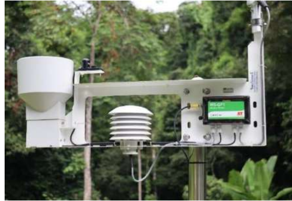
(F) Temperature, Humidity, Wind Speed, and Rainfall Measurement System at the Watershed Management Unit of Khun Kong
