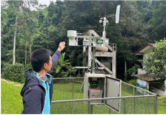
(F) Temperature, Humidity, Wind Speed, and Rainfall Measurement System at the Watershed Management Unit of Khun Kong
